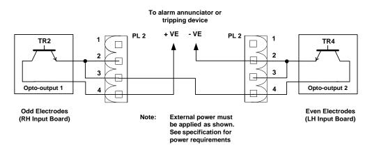
(Switch SW6 set for Fault Signal operation)
